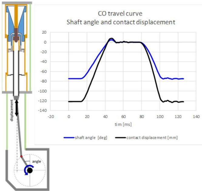
**Figure 6 - Example of travel measurement at the bell crank shaft.**
