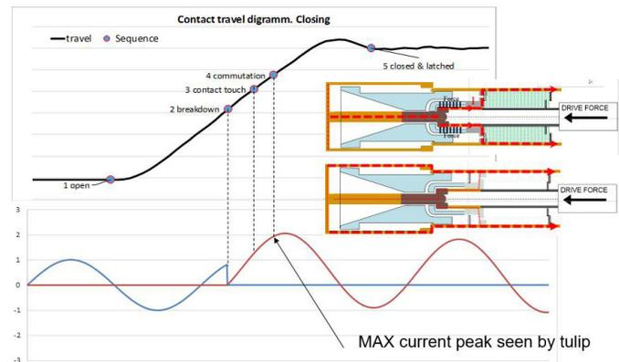
Figure 4 - Current making by closing operation.
