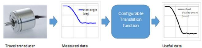
**Figure 8 – Principal data processing for getting the actual contact displacement**
