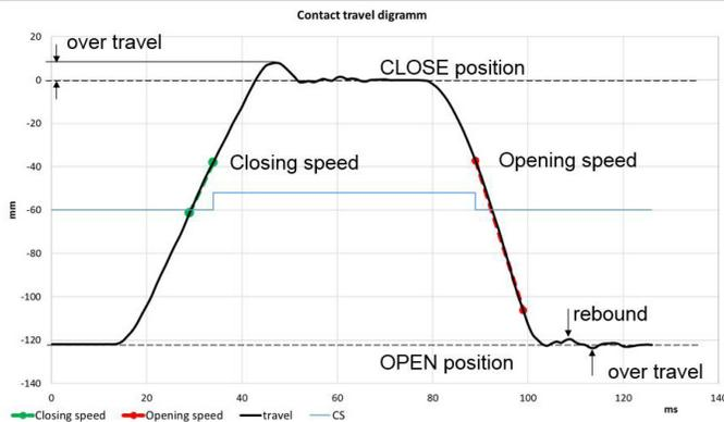
Figure 1 Typical travel curve for a CO operation. Main calculated parameters are:
