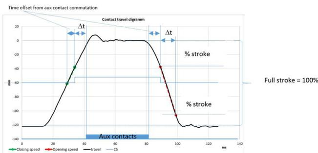
**Figure 9 – Travel curve speed evaluation**
