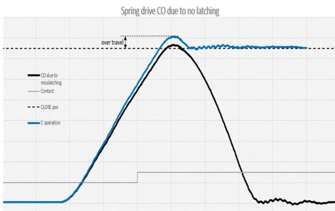
**Figure 5 - Travel curve of a circuit breaker with spring operating mechanism.**
