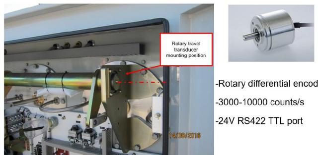
**Figure 11 - Rotary transducer**
